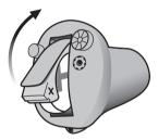
**Note:** Open the battery door fully to make sure the hearing aid does not drain the battery fully and to allow air to circulate whenever you are not using your hearing instrument, especially at night or for longer periods of time.
