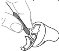
Open the battery door and turn the hearing aid so the lid is facing downwards (see illustration). Guide the short wax removing tool (no. 4) through the microphone openings on the door from the inside (see illustration).
