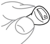
To turn the hearing aid on, close the battery door and push it upwards. The hearing aid will play a sound signal to indicate that it is on, unless your hearing care professional has deactivated this function.
